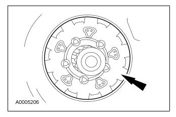
27. CAUTION: The low/reverse brake drum must be pulled forward to install the low/reverse planet retaining ring.
